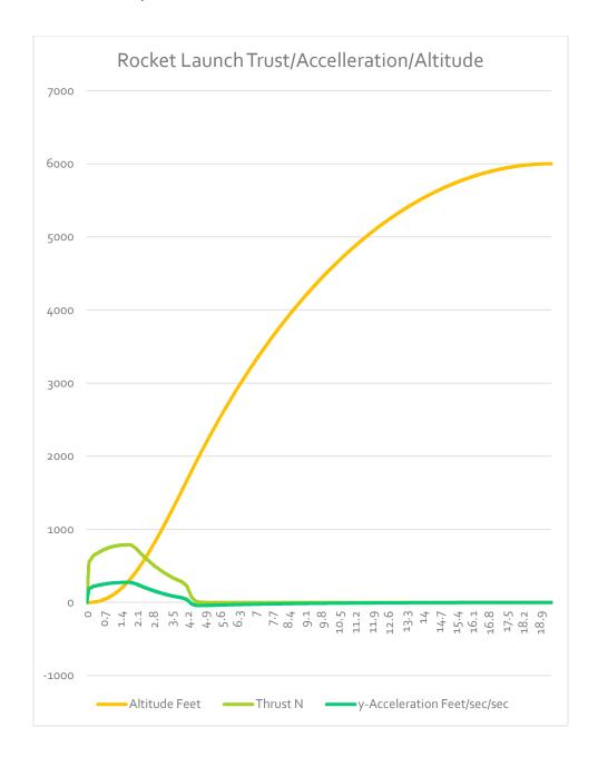
Our dimensions are 162.89cm long, and 15.87cm in diameter. According to Rocksim the rocket goes exactly 6,000 feet, but from our experience and knowledge Rocksim height estimate is about 20 percent low so according to our calculations the rocket should reach our target height, 5,280 feet. If the rocket does exceed the target height during initial testing, mass can be added to reduce the altitude of apogee.
